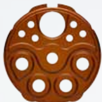
11-polig Buchse P Code 1 11-pin female contact P Code 1 (5 X Ø 2 mm (4 + PE) + 6 x Ø 1 mm)
